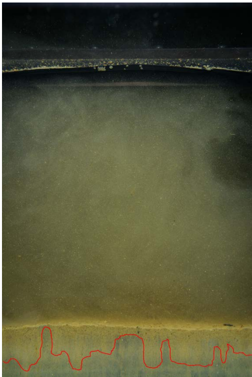
Underpenetration with Acceptable aRPD
