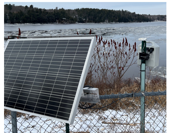
A camera (right) monitors ice blocks in a cove to help determine how ice could affect a cap, 2024.
