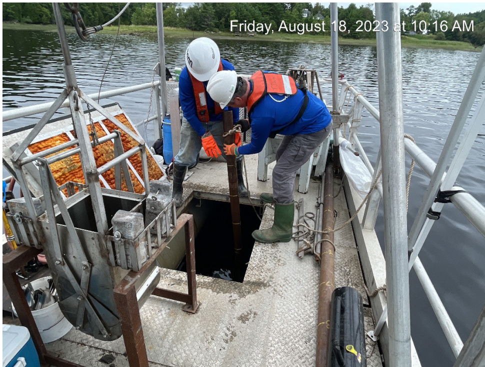
Photograph 41. Slam Bar in Use at OR-PDI-34 (August 18, 2023)
